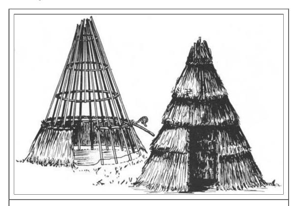
Figure 12: Yokuts conical house, central foothill type with mat door and inner ring at smoke vent. (After Rogers)
